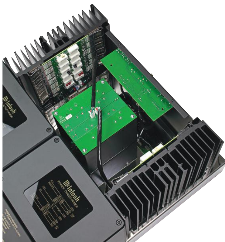
Internally, paralleled output transistors and their associated emitter resistors (white) sit on circuit boards attached to large heatsinks. This is a classic Class A/B amplifier, not Class D.
