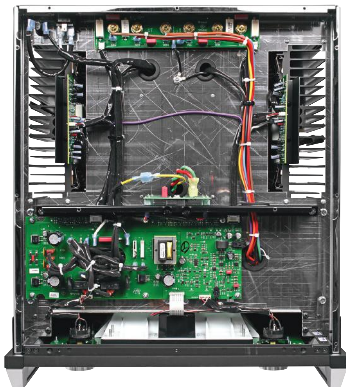
A stainless steel chassis supports the weight of the transformers, heavy coloured wires from the output auto-transformer, at right here, leading back to large gold plated loudspeaker binding posts at rear. There are no cooling fans so the unit runs silent.
